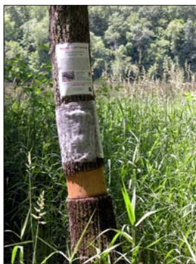
Detection tree construction
