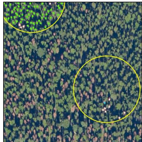
Figure 9. Screen shot showing process of digitizing live (green) and recently dead (red) trees in 1-acre circles on an orthophoto.
