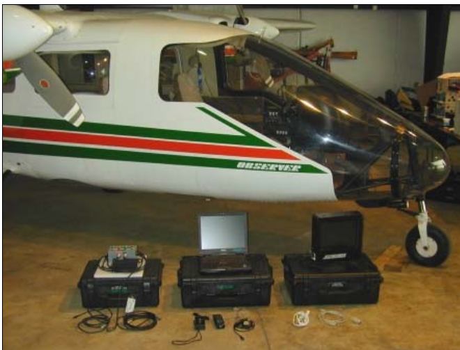
Specialized plane plus digital mapping equipment used during aerial surveys; photo by Keith Sprengel, USDA Forest Service.
