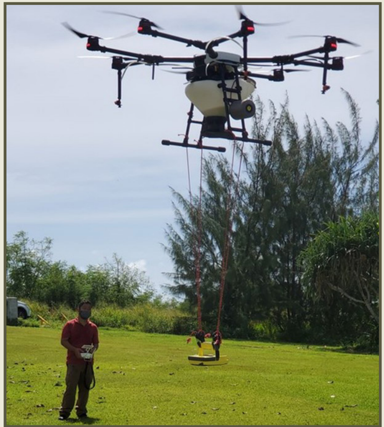
Figure 5. RECCO harmonic radar device suspended from an agricultural drone piloted by Glenn Dulla, Guam Department of Agriculture. Photo Credit: Aubrey Moore, University of Guam
