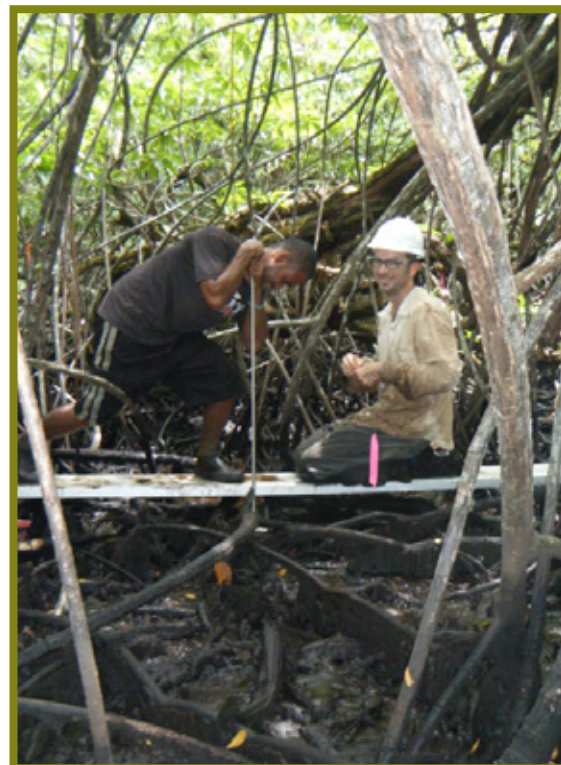
Figure 9. Installation of rod surface elevation tables in mangrove forests (Source: Richard MacKenzie).
