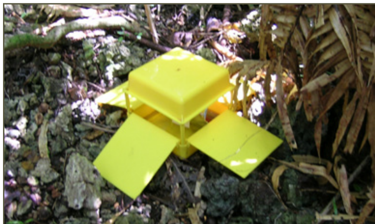
Ramp trap baited with pheromone lures of four species. Photo: Gadi Reddy, University of Guam
