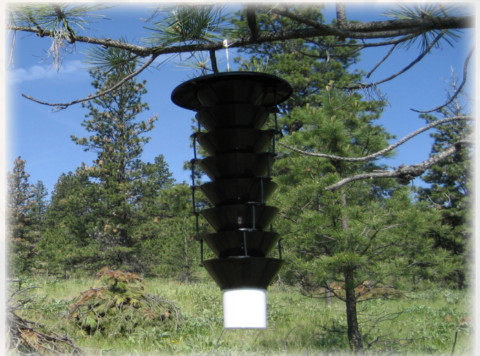
Early detection of non-native bark beetles involves hanging Lindgren funnel traps in at-risk forests
