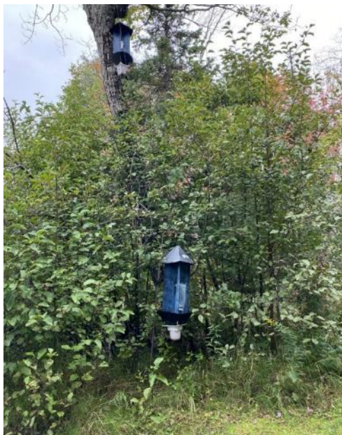
A cross-vane panel trap set near the ground and a second trap in the lower canopy of a tree at a research site.
