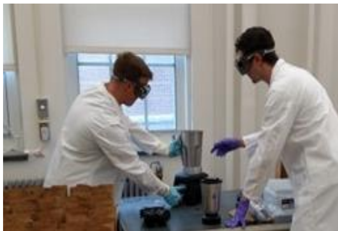
Connor Vanwagoner and Justin Keyzer grind hemlock needles for residue analysis using a commercial blender.
