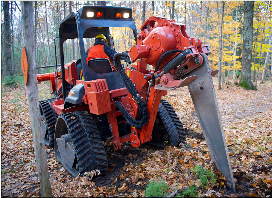
The vibratory plow blade used to treat infected stands of oak was specially designed and built at the Michigan Department of Natural Resources' Forest Fire Experiment Station in Roscommon. The plow cuts narrow trenches 5 feet deep to separate underground root systems, preventing further spread of the oak wilt fungus to uninfected trees.
