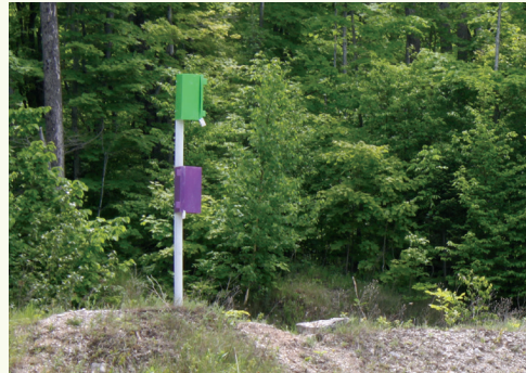
Double decker emerald ash borer trap with a green and purple prism.
