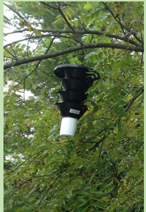
A Lindgren funnel trap, used to monitor for WTB.
