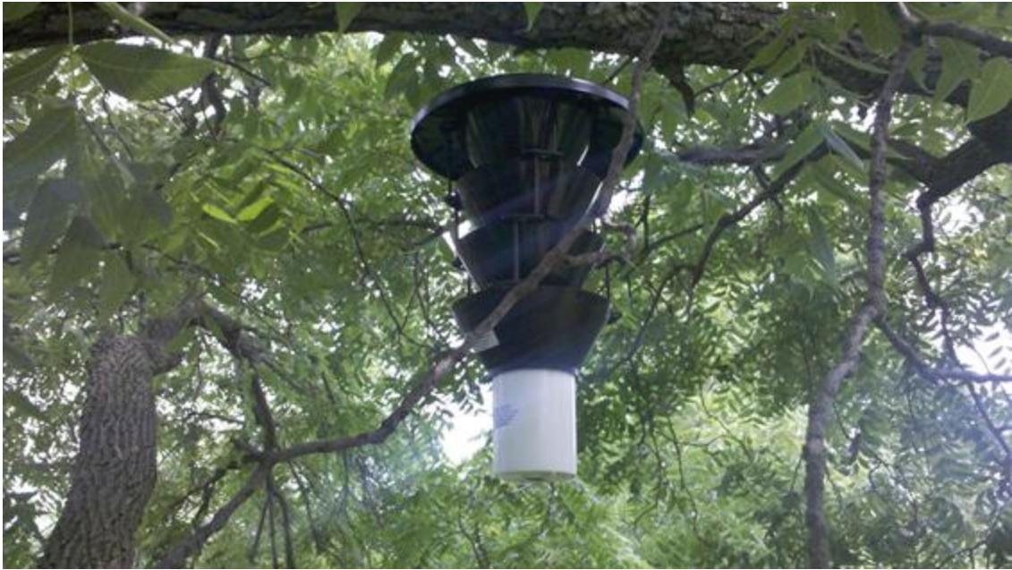
Figure 12. One of the Lindgren funnel traps that were used in conjunction with the walnut twig beetle pheromone. The traps were placed at sawmills, communities, and campgrounds. (Image: Shane Donegan, DNR)
