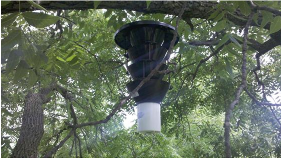
Figure 13. One of the Lindgren funnel traps that were used in conjunction with the walnut twig beetle pheromone. The traps were placed at sawmills, communities, and campgrounds. (Image: Shane Donegan, DNR)
