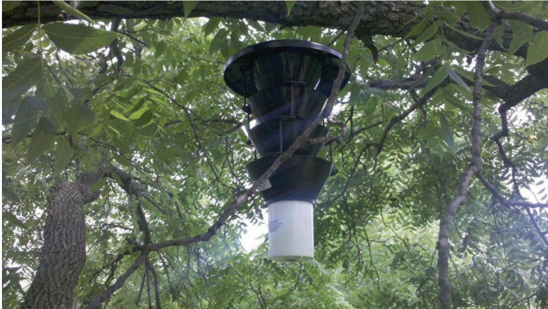
Figure 32. One of the Lindgren funnel traps that were used in conjunction with the walnut twig beetle pheromone. The traps were placed at sawmills, communities, and campgrounds. (Image: Shane Donegan, IDNR)
