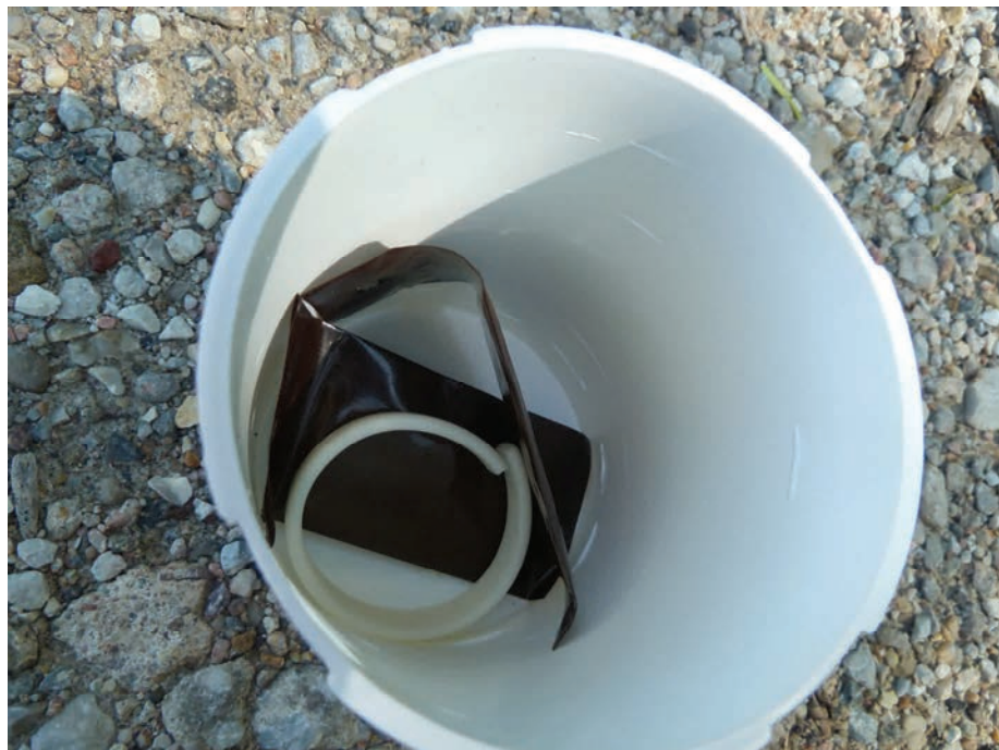
Figure 33. A look inside the Lindgren Funnel trap capture chamber. The picture shows two pheromone pouches and a 3 inch long strip of dog collar that was used to kill the beetles that entered the capture chamber. (Image: Shane Donegan, IDNR)
