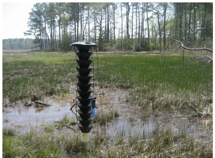
A Lindgren funnel trap is set up as part of the Southwide Southern Pine Beetle Pheromone Study.
