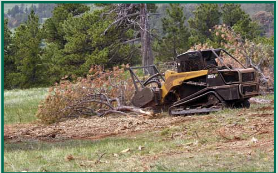
Roller-choppers are used to convert infested trees into wood chips and destroy MPB broods.
