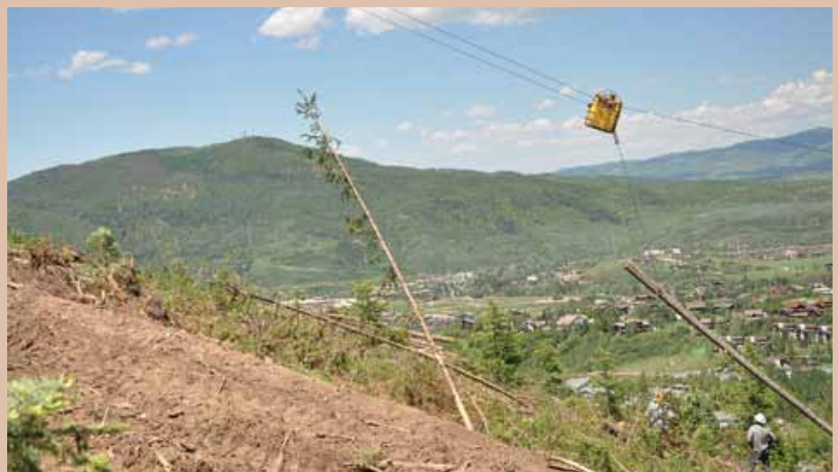
Dead and downed trees were removed from areas around Steamboat Springs using cable logging equipment. (Photo by Kathryn Hardgrave)
