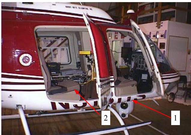
Figure 14. TIR Data collection system mounted on a Bell JetRanger Helicopter. A gyro-stabilized mount containing the FLIR and the visible band color video camera is attached to the underside of the helicopter (location1). A computer, global positioning system (GPS), and digital video recorder are mounted on an equipment rack in the back seat (location 2).
