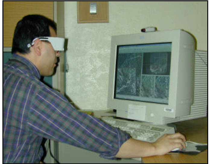
Figure 4. A photo interpreter viewing in stereo with the aid of glasses that mimic the screen flicker. Combining real time GPS control and forward motion aerial photography, with software and hardware capable of orthorectifying, zooming into a photo and viewing in stereo, provides the key for precisely and accurately measuring individual trees and deriving other pertinent information.
