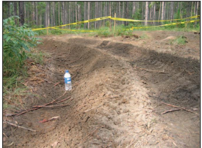
Figure 54—Loop B, 8-inch rut on the turn.
