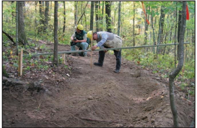
Figure 44—Rut depths of 1 to 4 inches were recorded.
