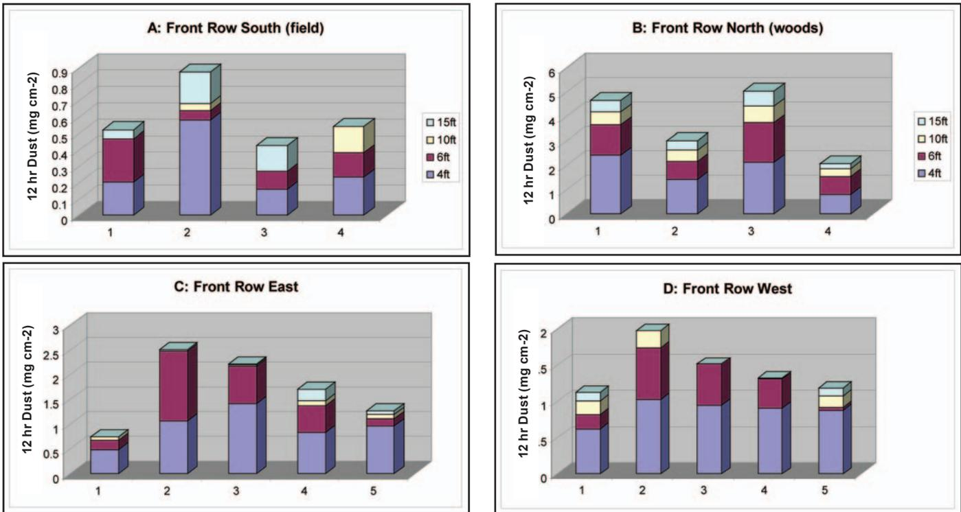
Figure 9—Dust accumulation on passive samplers after 10 hours. Each bar indicates one sampling pole and the divisions indicate the quantity of dust collected at each sampling height.
