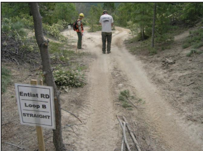
Figure 81—Loop B straight after 960 passes.
