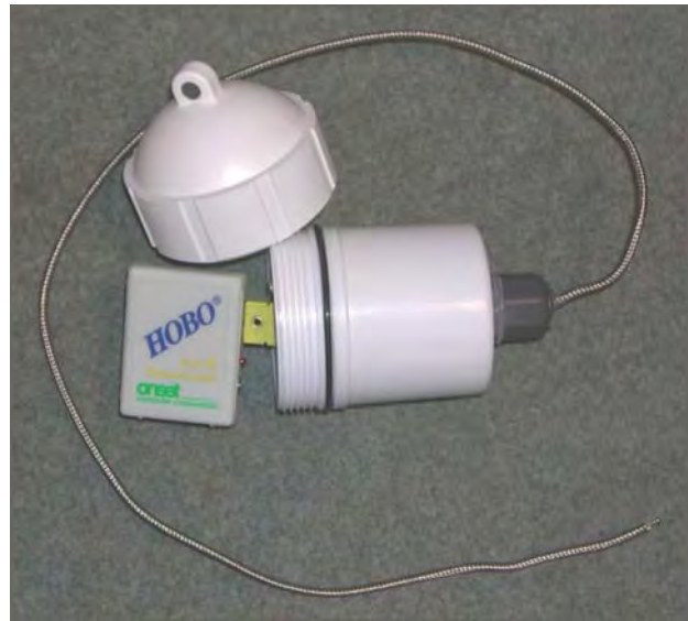
Figure 5. Firelogger showing HOBO datalogger, white plastic case, and thermocouple wire
