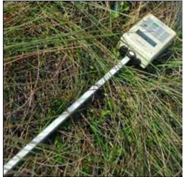
Figure 3. Decagon Ceptometer for measuring light to estimate biomass.
