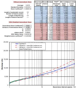
**Figure 1:** Example flow frequency analysis results for 131 years of systematic record for the Cache la Poudre River (Example Computation Sheet 2, in spreadsheet).
