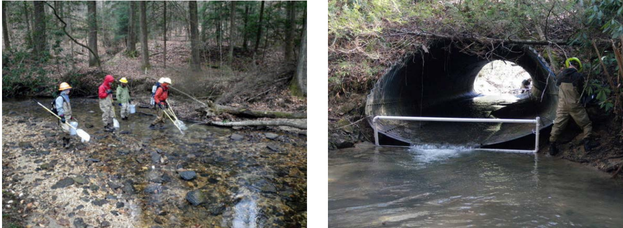
Figure 1: (On left): Mark/recapture of individual fish using backpack electroshocking. Figure 2: (On right): Stationary Antenna PIT tag monitoring at a “Gray-Moderate” road-stream crossing. Credit: Craig Roghair, Center for Aquatic Technology Transfer, USFS
