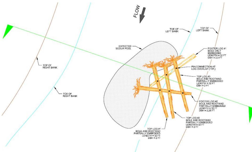
Figure 6: Sample multiple log structure layout (not to scale).
