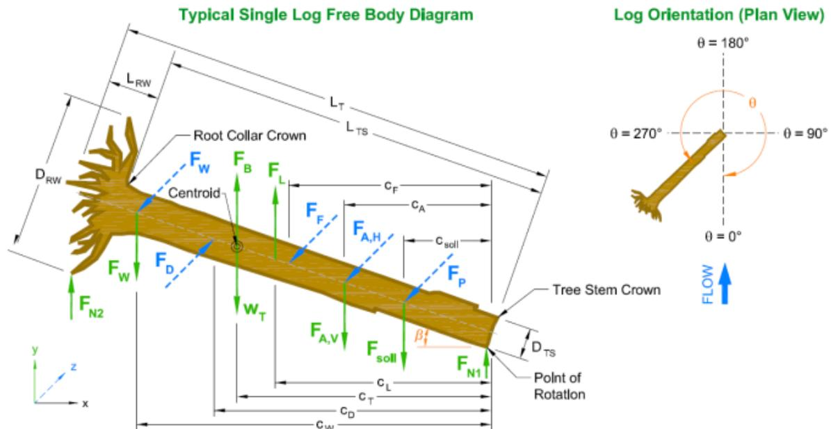
Figure 1: Typical Single Log Free Body Diagram and Log Orientation.
