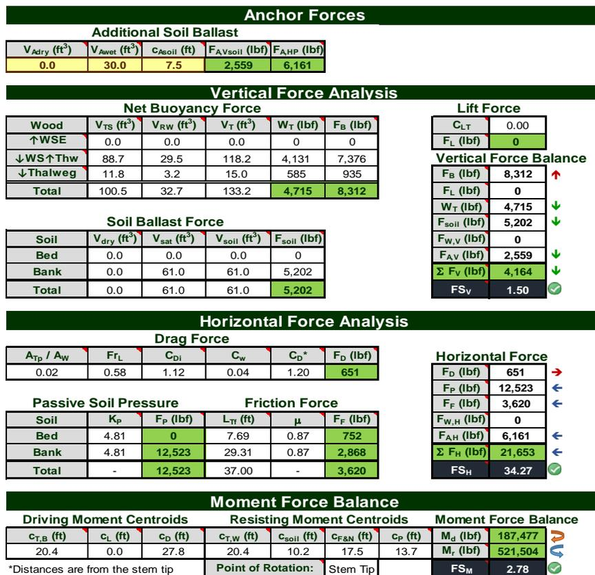
**Figure 5:** Model output of force balance analysis for the single log structure.
