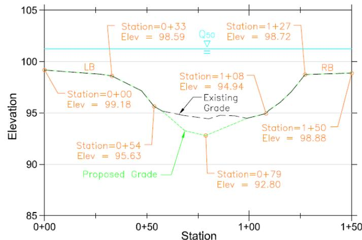
Figure 7: Sample multiple log structure cross section
