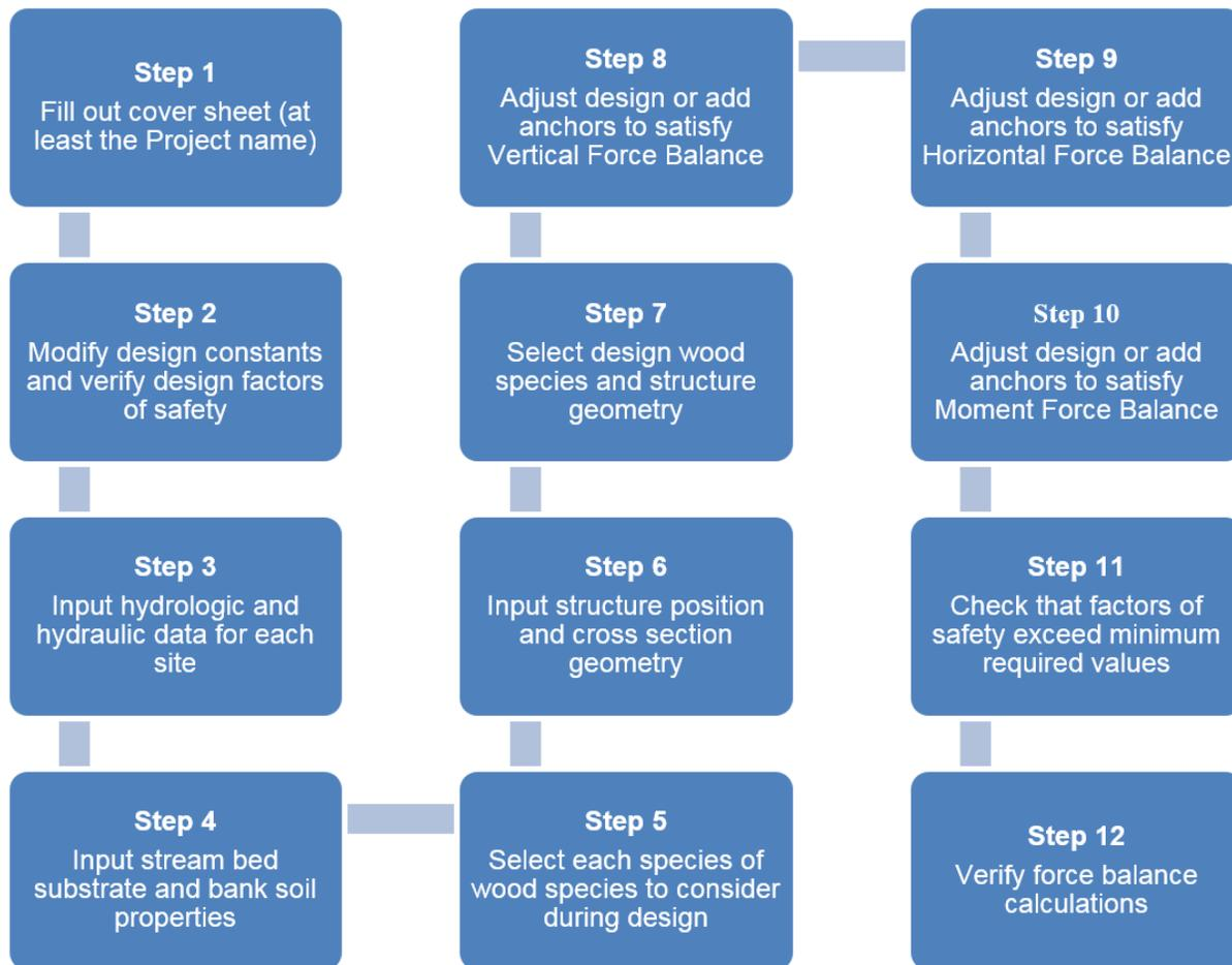
**Figure 3:** Single log structure design procedure.
