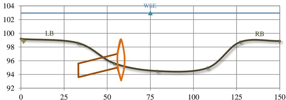
**Figure 4:** Model output of the single log structure cross section.
