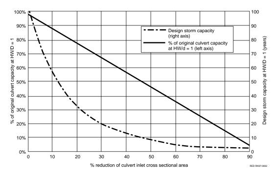
Figure 4—The percentage of cross sectional area reduced by crushing or partial plugging of the inlet is nearly equal to the percent of hydraulic capacity reduced (solid line). However, these reductions in capacity translate to large reductions in design storm capacity (dashed line). In this example from northwest California, a culvert originally sized for the 100 year design storm at HW/d=1 can only pass the 25-year storm with a 25 percent reduction in cross sectional area.
