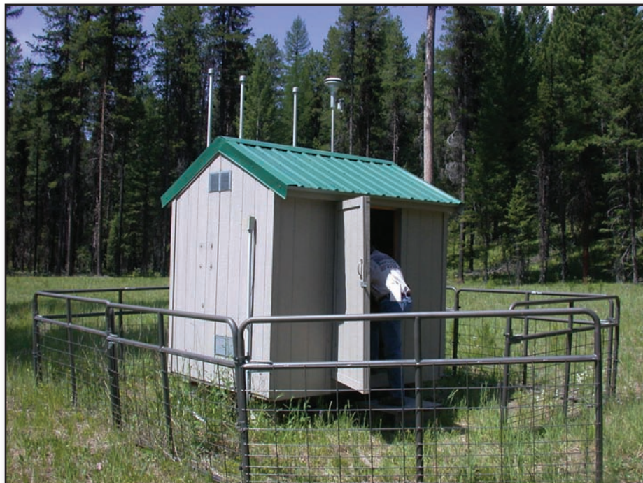
Figure 37—Monture Guard Station IMPROVE site (MONT1), Lolo National Forest. This site is slightly influenced by emission sources in the Bitterroot valley, particularly Missoula. This site houses four modules that pump air in 24 hour periods on Wednesdays and Saturdays. Filters are changed each Tuesday then sampled for a wide variety of chemical air quality constituents. A visibility camera associated with the site is located at Ovando, Montana.
