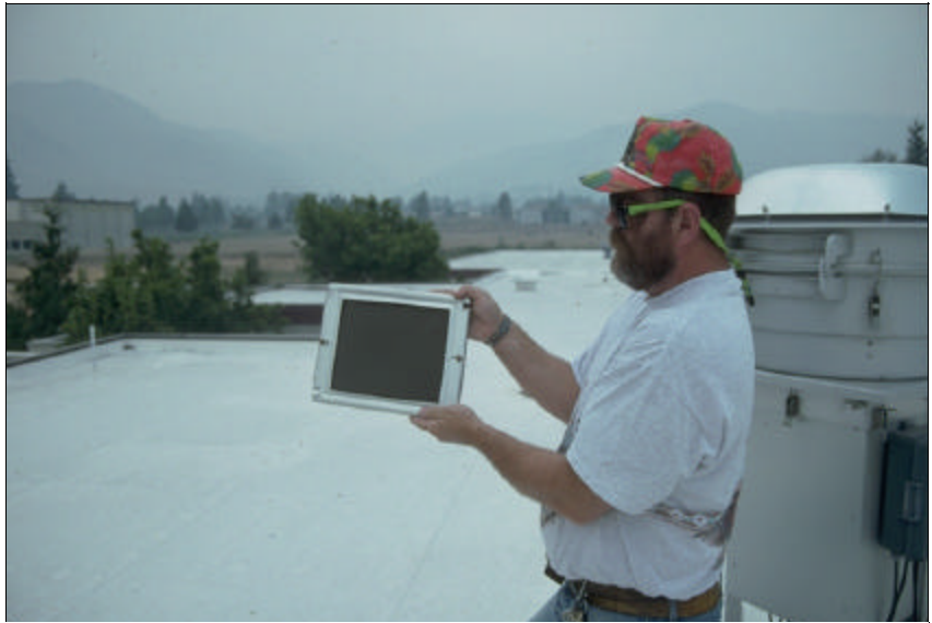
Figure 21 — PM10 filter taken in Wenatchee, WA during impacts of emissions from a wildfire. Since the filter was clogged, the data was not included in the States emission database. The filter clogged @ 300+ Ug/m3.
