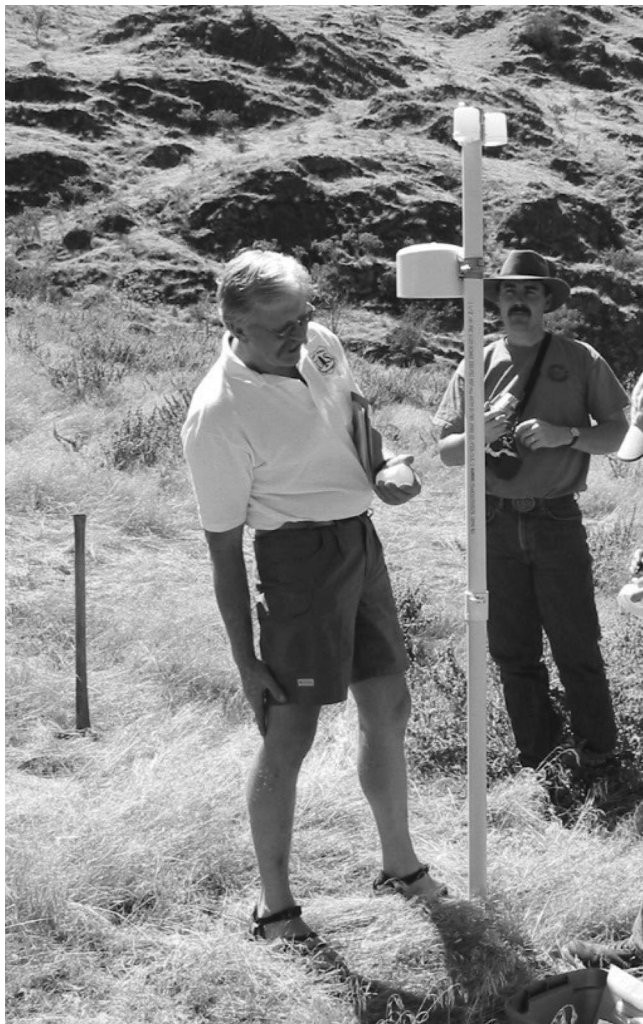
Figure 2. The passive sampling station at Kirkwood Ranch. The large inverted cup shelters the Maxxam samplers; small cups shelter the Ogawa samplers.
