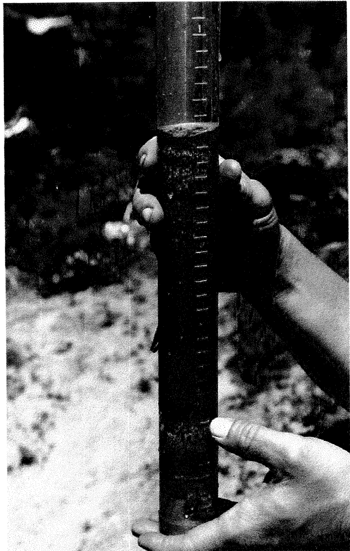
Plate 7. Sediment core from Gertrude Lake. Increments of 1 cm are inscribed on the core tube.
