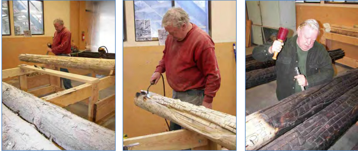
Figure 4. Hal Payne creating posts and caps for Nicholson Adit portal. From left to right: Shaping the log from historic photos, charring the outside of the log to give it the correct color and putting on the finishing touches.
