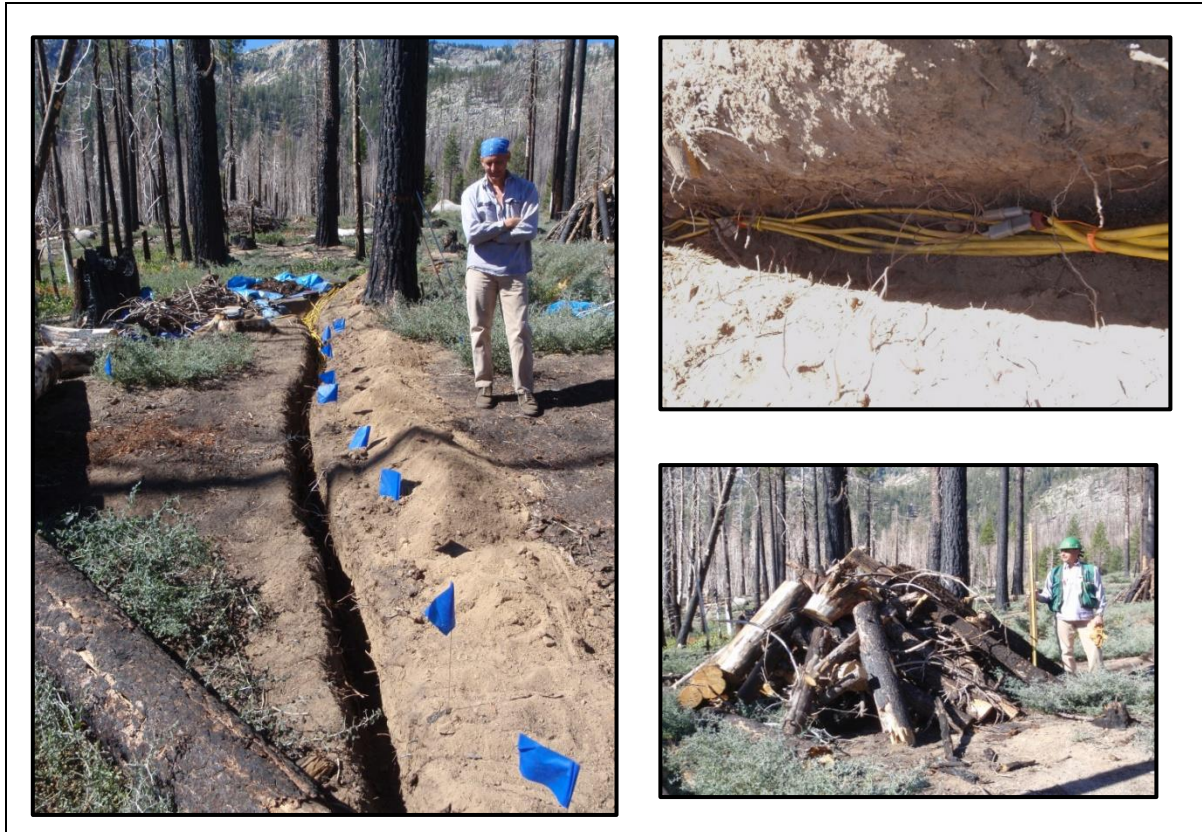
Figure 8. Testing spatial variability in soil heating at the Angora site (pile #1). Pin flags in the photo on left identify the location where heat-sensing thermocouples were installed. Thermocouples attached to datalogger cables (top right photo) were placed horizontally in undisturbed soil at 5- and 10-cm depths before the pile was reconstructed (bottom right photo).
