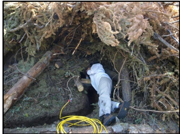
Figure 6. Deconstructing about one-half of a pile (Sugar Pine #1) and installing thermocouples wires at the pile center. Thermocouples were placed horizontally at specified depths in undisturbed soil (right photo) before reconstructing and burning the pile.
