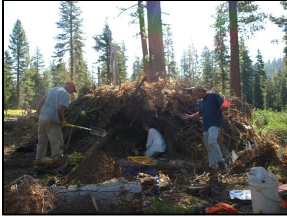
Figure 6. Deconstructing about one-half of a pile (Sugar Pine #1) and installing thermocouples wires at the pile center. Thermocouples were placed horizontally at specified depths in undisturbed soil (right photo) before reconstructing and burning the pile.
