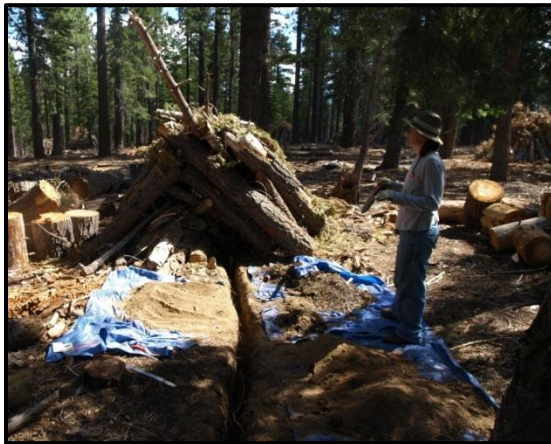
Figure 7. Thermocouple cables were placed in 30 cm-deep trenches (left photo) that extended well beyond the pile edge to avoid heat damage to the dataloggers. The photo on the right shows a completed pile at Washoe State Park, with thermocouples installed and the trench back-filled with soil.
