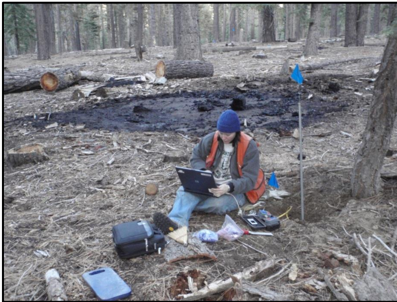
Figure 15. Downloading soil temperature data from the “mopped-up” pile in the background at Washoe State Park. This pile was lit at approximately 0900 and mopped-up at 1700, with ~95% of the pile consumed within 8 hours of ignition. Similar consumption was found for all piles receiving water mop-up.
