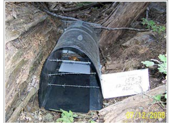
A fisher trap. As a target species (e.g., fisher, gray fox [ Urocyon cinereoargenteus ]) enters the track-plate enclosure to inspect the bait (chicken, at the rear of the enclosure), its feet collect soot from the dark track plate and deposit tracks on the light adhesive surface (Contact® paper) positioned just in front of the bait. Animals are prevented from entering the back of the track-plate station by fastening a piece of mesh hardware cloth to the rear of the box. The barbed wire positioned near the entrance to the enclosure often collects hair from larger target species as they enter the box to inspect the bait.
