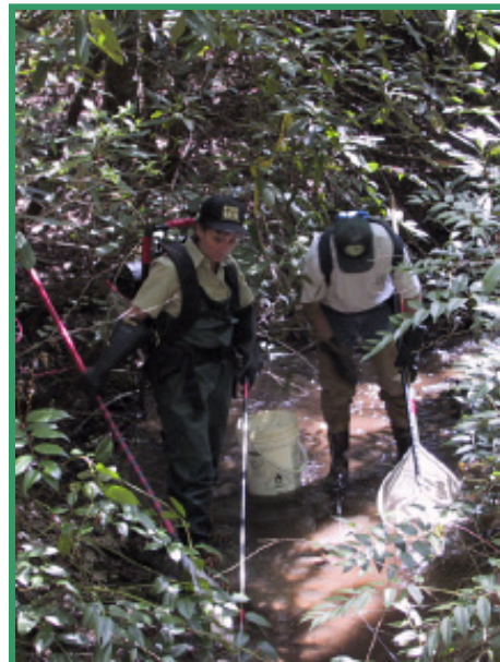
Figure 8 – Monitoring Streams using Electro-fishing
