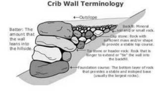
4) Building the wall- While laying your courses, concentrate on splitting the gaps or breaking the joints. This means laying your next rock directly above where the two rocks below it meet. Think of a brick wall. Take your time and find the rock that fits without any teetering. Move the rocks around and if it isn't working, start over and try different combinations. A little patience now
