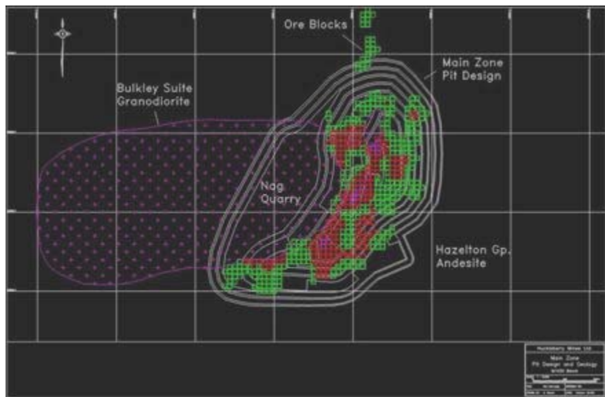
Figure 6.7 Geological block models are used in most mines for mapping environmental geochemical information.
