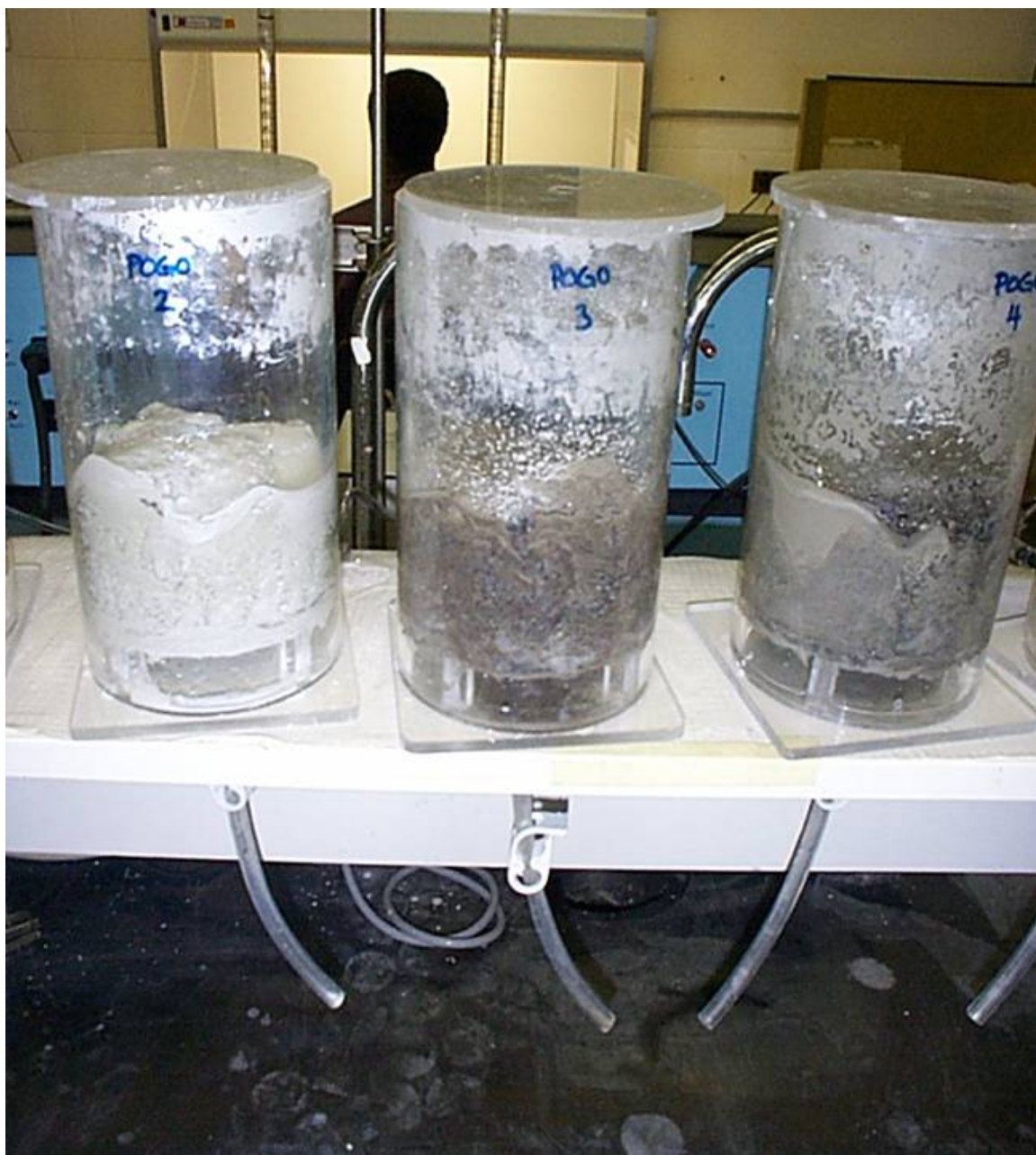
Figure 18.3 Photograph of humidity cells being used for waste rock.
