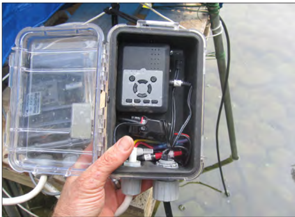
Close up of the mDVR used in fish monitoring. Photo by Thor Eide.
