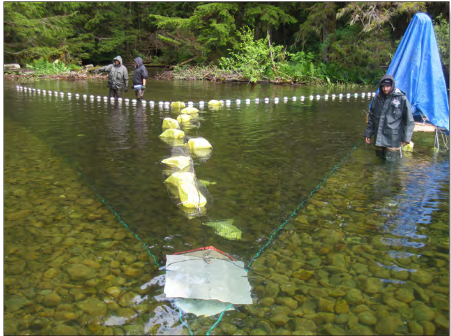
Cameras film fish traveling through net weirs. Photo by Ben VanAlen.
