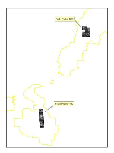
By using the historic map supplied, OR\_Umatilla\_south\_1936.tif, TTEC was able to digitize the section lines from the map and use this to compare positional accuracy for 11 positions between the map/coverage polygons and the photo (see figure of example below)
