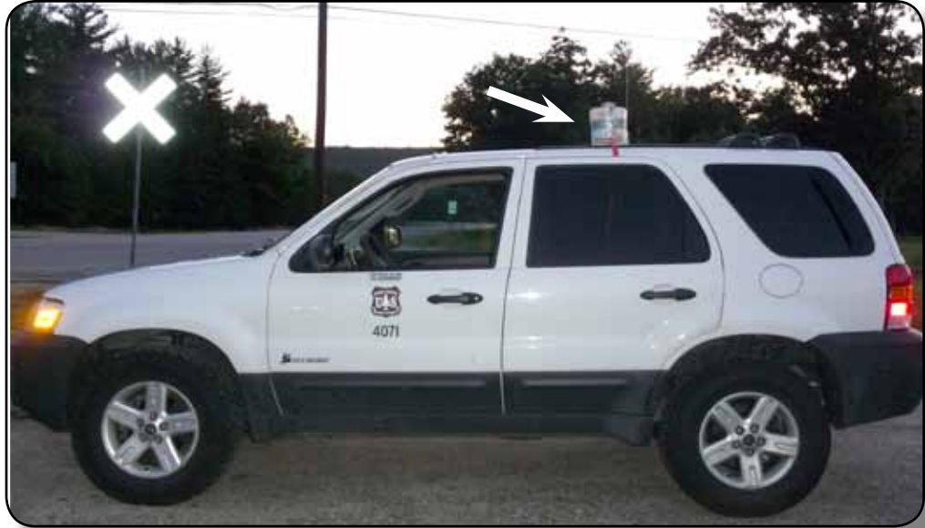
Figure 32. Forest Service vehicle equipped with Anabat bat detector in a watertight container on the roof. WMNF photo by Leighlan Prout.
