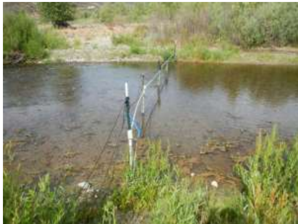
Photo 11. PIT tag antenna array spanning the Scott River just upstream of the mouth of French Creek, 6/19/14 (RCD).
