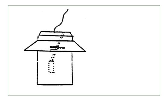
Step 6—Fold the top ends of the trap in toward the center of the trap so the two sides are parallel to one another.
