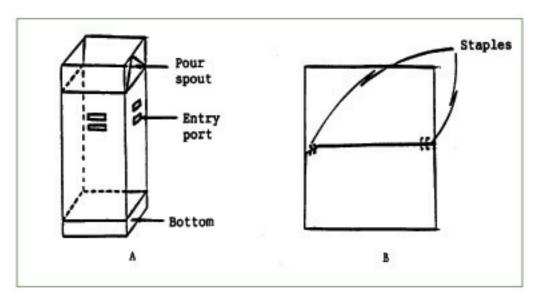
Step 3— Pop out the center insert of the trap hood, crease all tabs up, and crease all solid lines.
