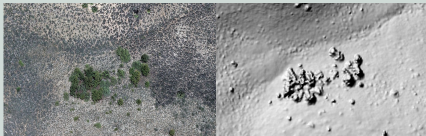
Figure 8—Subset of the 10-cm imagery ( left ) and a hillshade ( right ) created from the 10-cm imagery and ERDAS eATE.
