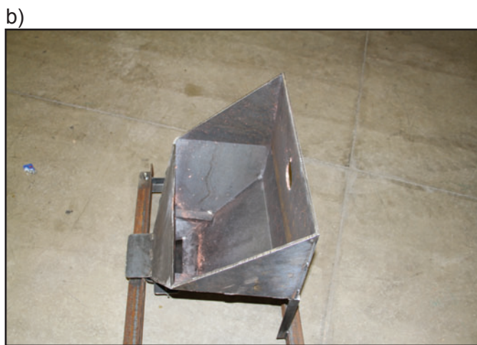
Figure 9 —Photographs of the “birdhouse” attachment to the deflector plate on the bullet trap that allowed collecting and concentrating fragments onto plates painted with temperature sensitive paints: (a) Front view showing hole through which the bullet passes, (b) side view showing baffles and funnel, (c) top view showing location of plate in the bottom of the funnel.
