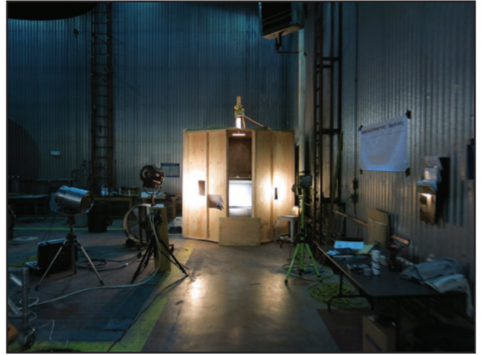
Figure 7 —Bullet trap was housed in a plywood shell to shield laboratory equipment from stray fragments. Windows were cut in the doors for lighting and cameras.
