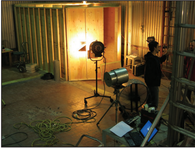
Figure 7 —Bullet trap was housed in a plywood shell to shield laboratory equipment from stray fragments. Windows were cut in the doors for lighting and cameras.
