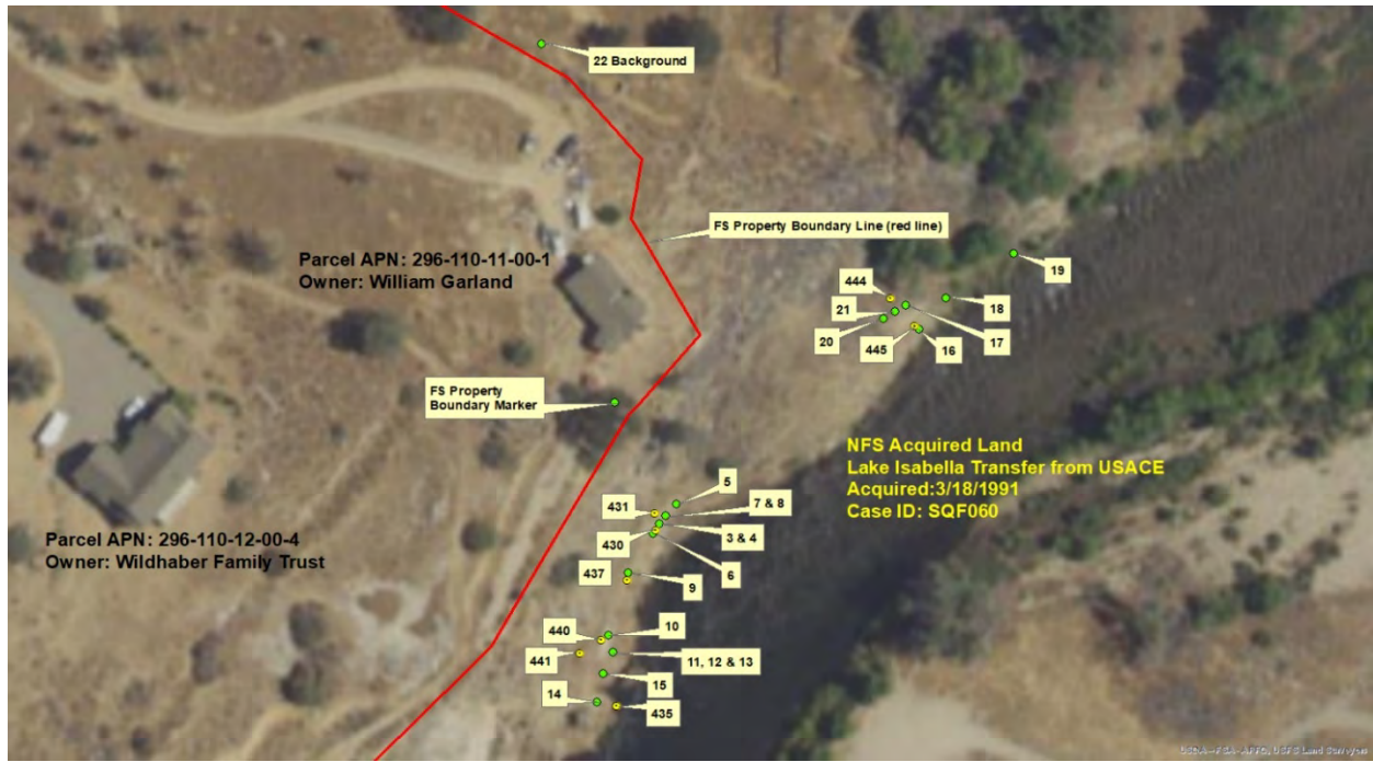
Figure 14: January 14, 2020, XRF (sample Locations 429-445 taken by the Thermo Scientific Niton Model XL3t-600 and sample numbers 3-22 by the Olympus Delta XRF Model DS-4000).
