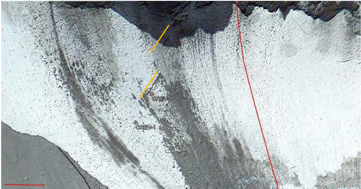
Figure 8. Close up of Crev-1 points surveyed in September 2015 overlaid onto 2013 Google Earth image. Comparing Figure 8 to Figure 7, the stepwise crevasse in the Figure 8 image is likely the en echelon fracture pattern of the incipient opening of the bergschrund seen in the 2015 photo (Fig. 7). Red scale bar in lower left is 20 m.
