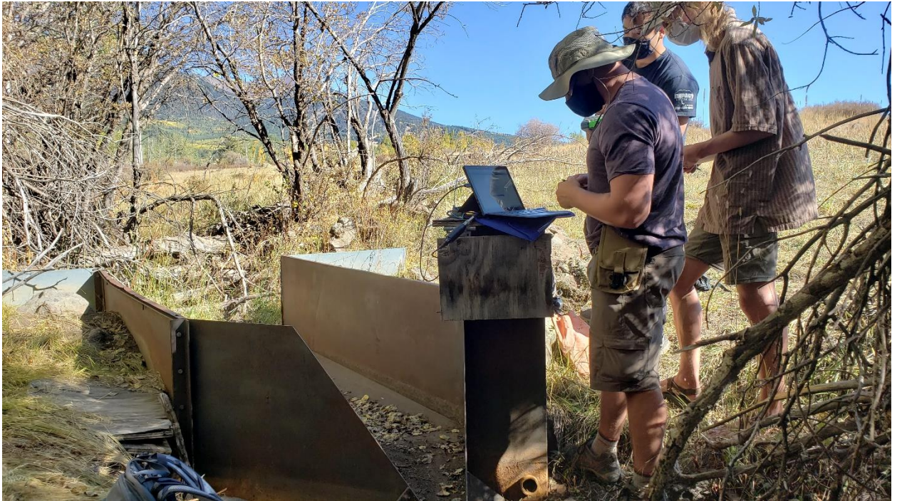
Figure 4. Maintaining Hart Prairie flume and downloading data logger in October 2020.
