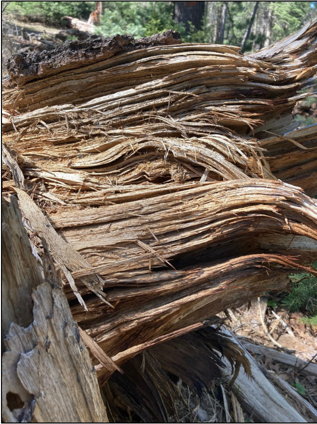
Figure 31. Laminated decay, a type of white rot where the wood separates at annual growth rings.
