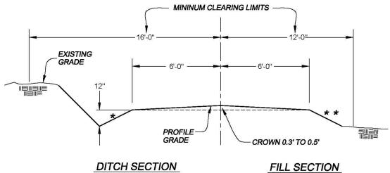
\*BACKSLOPE AND DITCH SLOPES MAY VARY FROM 1H:1V TO 2H:1V WHEN CUTS ARE UNDER 2 FT. CUTS OVER 2 FT. SHALL HAVE SLOPES OF 2H:1V
