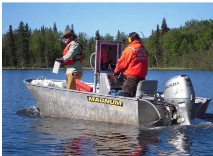
Figure 54. Liquid herbicide being applied into Beck Lake from two trailing hoses on either side of the stern. Note the pump system hanging from the aft side of the center console; the mixing tank is immediately below. Containers of undiluted herbicide are stored in the bow. Photo by John Morton.
