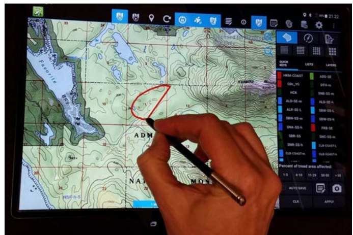
Figure 88. The current sketch-mapping tablet and DMSM software aid aerial survey data collection.
