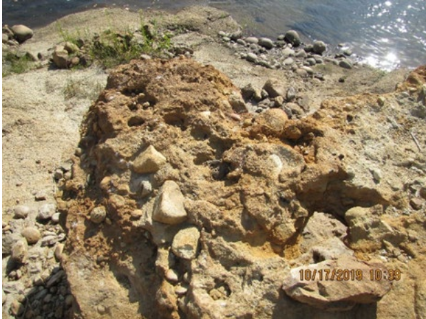
Figure 11: Rust colored tailings and mineral processing deposits along the Kern riverbank below the former mill.
