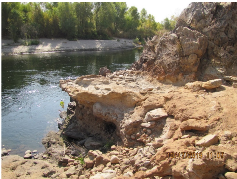
Figure 12: Deposits of very fine white powdery material along the riverbank (left) and brown silty materials below the former mill foundation (right) where elevated arsenic, lead and mercury were found.
