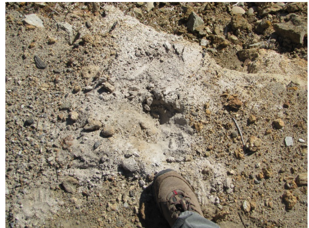
Figure 12: Deposits of very fine white powdery material along the riverbank (left) and brown silty materials below the former mill foundation (right) where elevated arsenic, lead and mercury were found.
