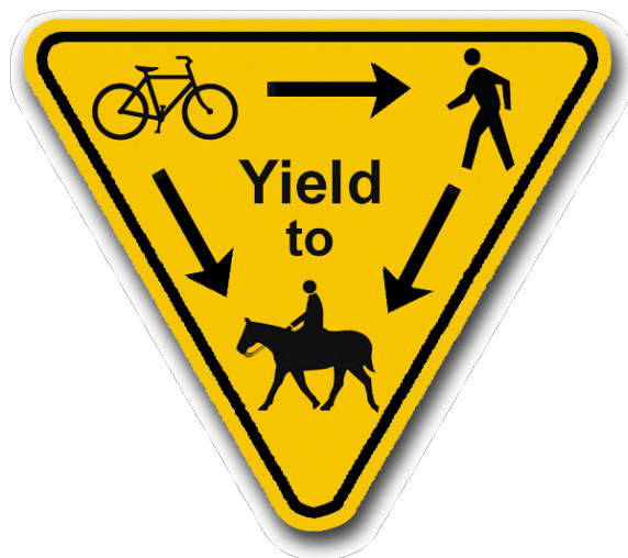
Figure 43. Trail courtesy “Yield Triangle” graphic typical of trail signage for multiple-use trails
