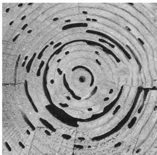
FIGURE 28.—Cross section of wood damaged by western subterranean termite ( Reticulitermes hesperus ), showing preference for springwood.
