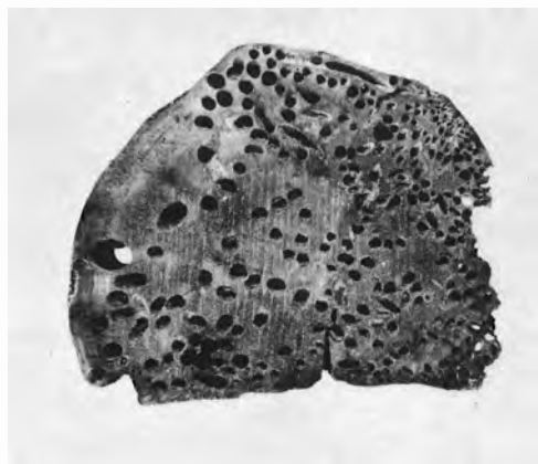
FIGURE 10.—Cross section of log honeycombed by shipworms, mollusks in the family Teredinidae.
